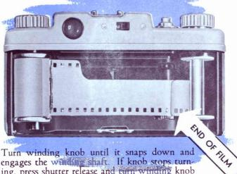
Turn winding knob until it snaps down and engages the winding shaft. If knob stops turning, press shutter release and earn winding knob until end of film lies back against the sprocket.
