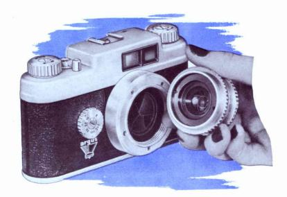
The Cintar f:3.5 lens on the Argus 21 is removable, and may be used on an enlarger. Unscrew the lens by means of the knurled ring at the base of the lens mount, adjacent to the camera. Do not unscrew by means of the focusing ring or focus adjustment may be damaged. There is no danger of fogging film in the camera when the lens is removed.
