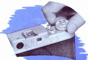
Make it a practice to wind the film by turning winding knob as far as it will go just before taking a picture. This will prevent tripping the shutter release accidentally. The counter indicates pictures left on the roll. The shutter is automatically set for the next picture when the film is wound. Thus, you cannot accidentally take two pictures on the same film.
