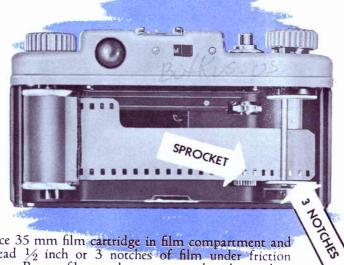
Place 35 mm film cartridge in film compartment and thread ½ inch or 3 notches of film under friction roller. Be sure film notches are engaged with sprocket. Follow illustration closely.
