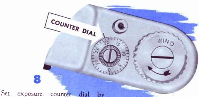
pushing down with thumb and turning clockwise until index line is opposite 20 or 36, depending on film used. The camera is now ready for the first picture. The counterdial will indicate at all times the number of pictures left on the film.
