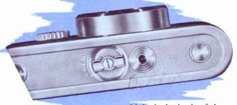
Unlock the back of the camera by turning the locking catch on the base of the camera in the direction marked "open".
