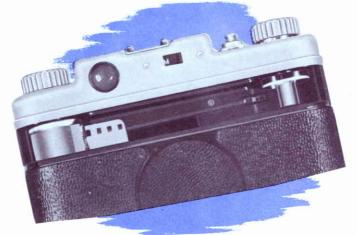
Replace camera back making sure it is fully closed and the locking catch turned to the locking position.
