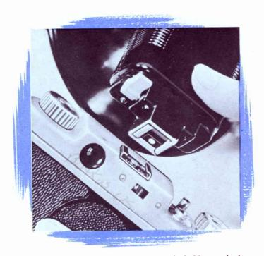
Argus 21 may be used with the Argus Flash Unit, which clips to the top of the camera. Synchronization is built into the camera and is correct at all shutter speeds. For complete information refer to flash unit instructions.
